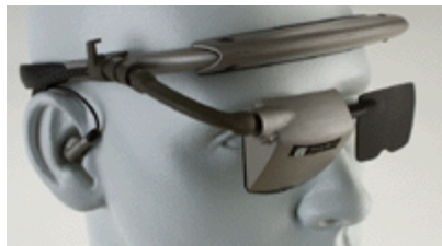
Virtual Vision eGlassII Single Display, Video See-Through HMD Courtesy of Microvision, Inc. 2002 Used with permission
