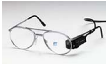
Figure 7 MicroOptical Clip-On Monitor Courtesy of MicroOptical Used with permission
