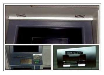
Skimming typically involves the use of hidden cameras (top) to record customers' PINs and phony keypads (right) placed over real keypads to record keystrokes.
