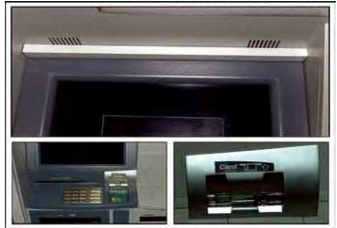
**Skimming typically involves the use of hidden cameras (top) to record customers’ PINs and phony keypads (right) placed over real keypads to record keystrokes.**
