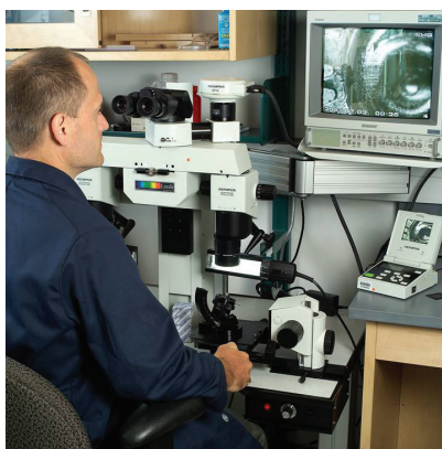
FTU comparison microscope makes it possible to observe two specimens simultaneously. The monitor next to the microscope displays the image.
