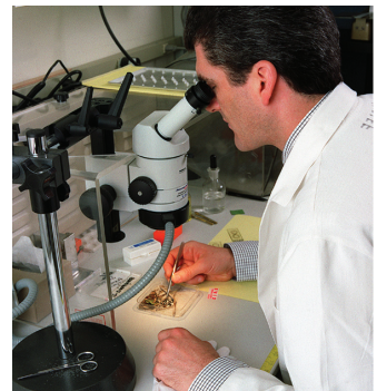
The stereo binocular microscope is routinely used for the preliminary analysis of trace evidence.
