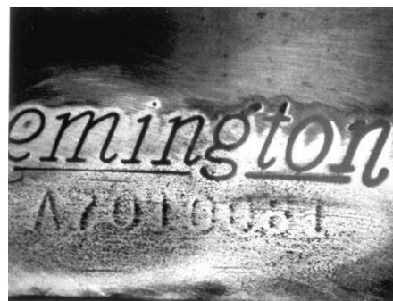
FTU serial-number restoration: On steel firearm frames/receivers, the serial number is restored using a mixture of magnetic shavings and oil.
