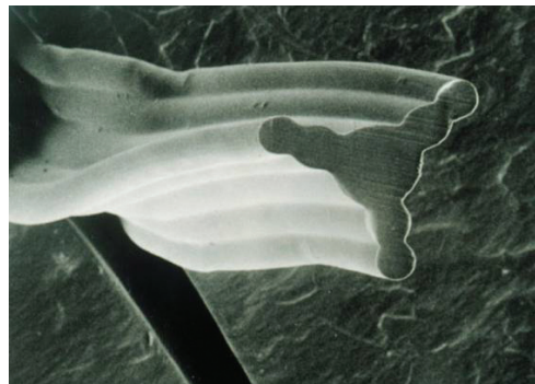
An electron micrograph of a cross section of a trilobal carpet fiber recovered from an automobile
