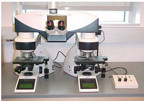
The comparison microscope is routinely used for side-by-side comparison of hairs and fibers.
