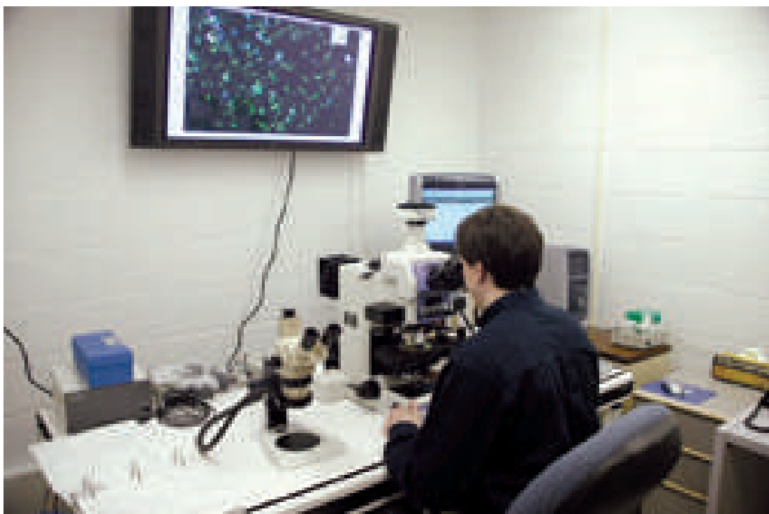
A Visiting Scientist evaluates the use of cathodoluminescence as a means of determining the geographic origin of mineral grains. The resulting information could be used as a point of comparison in forensic examinations involving soil, building materials, and other geologic material.
